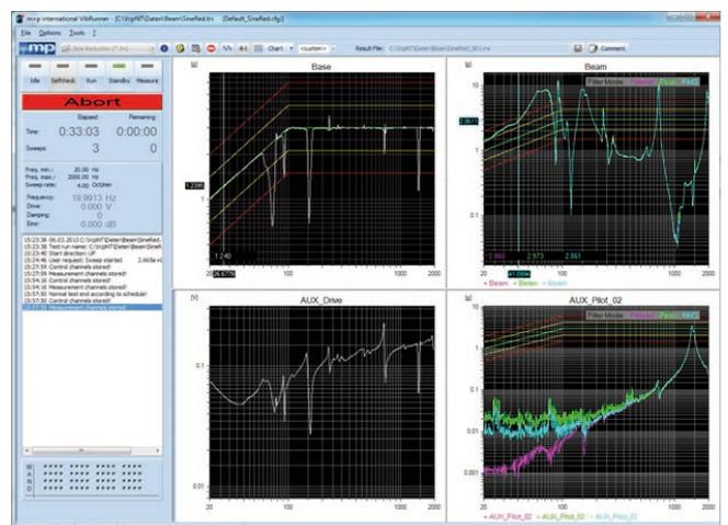
Online data reduction during closed-loop sine vibration test
