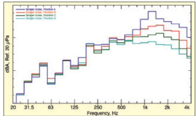
Figure 7. Noise measurements on station platform from each test point on slab.
