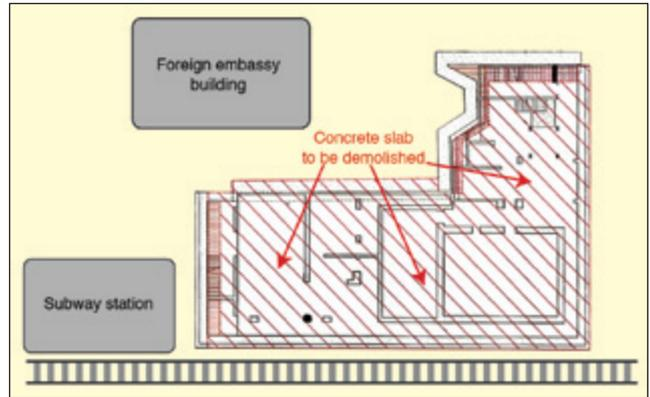
Figure 1. Location of slab showing nearby structures.
