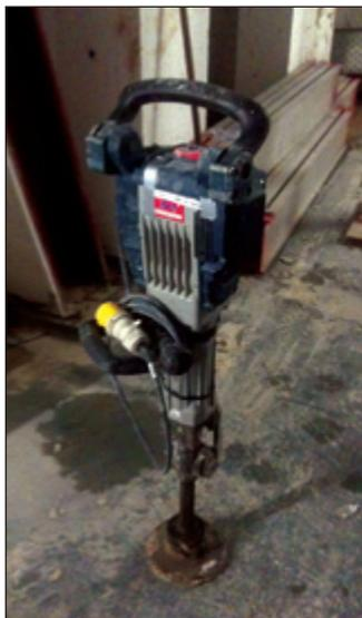
Figure 6. Mechanical tamper used during noise measurements.
