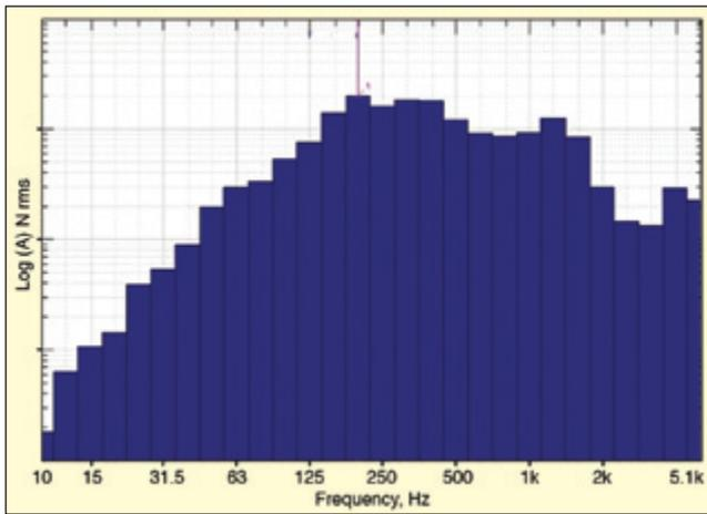
Figure 4. Calculated force spectrum for breaker tool.
