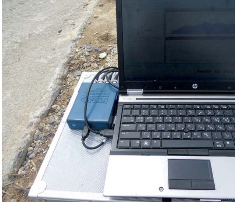
SO Analyzer with 4-channel NI 9234 CompactDAQ acquisition instrument
