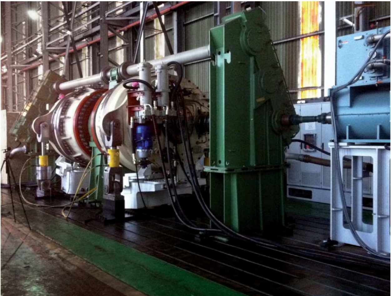
Wind turbine gearbox testing at Doosan Corporation Mottroll, South Korea
