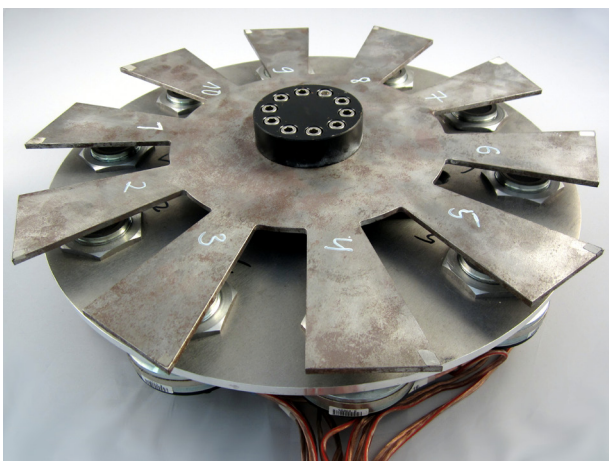
Figure 3a: Experimental setup consisting of 10 rigidly clamped loudspeakers and a simplified blisk
