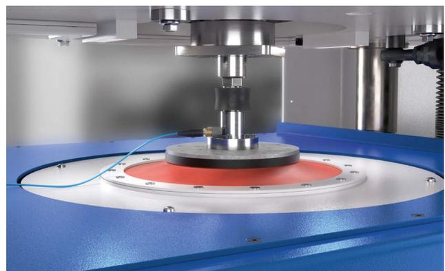
m+p VibControl is also used in the **HFe 3** high-frequency test rig to determine the dynamic stiffness of elastomer mounts. The electrification of vehicles has brought into focus new types of annoying cabin noises, which have so far been masked by combustion engines. Especially for elastomer mounts used in electric and fuel cell vehicles, the HFe 3 offers a way to future-proof your design through vibration tests at high frequencies up to 3 kHz and preloads up to 8 kN.
