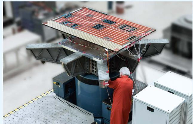
functions such as alarm and abort limits as well as notching. With force limiting, you prevent over-testing in critical frequency ranges.
